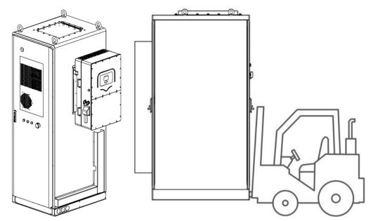
The battery racks should be moved to the designated position by means of forklift transfer or lifting, and the lifting ear should be re-checked and painted up if necessary.
