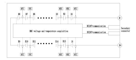
Electrical schematic diagram of battery module
