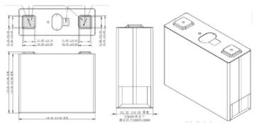
The standard 100Ah Lithium Iron Phosphate (LFP) square aluminum shell cell is manufactured by a fully automated production line. This cell performs excellently in continuous power, high cycle life, high storage life and high safety. The table 1 shows cell's basic parameter.
