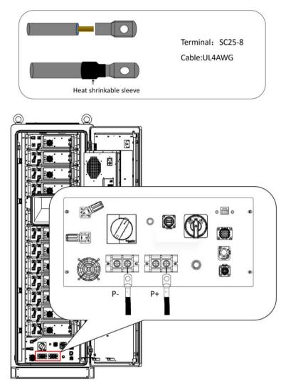
Connecting the P+ and P- Terminals to the DC Side of the Three-Phase Inverter.
