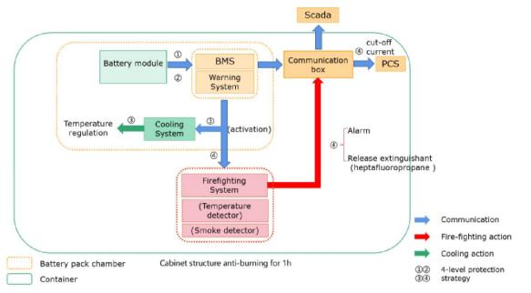
The system considers natural decay, abnormal charging and discharging, early internal short circuits and thermal runaway etc. based on 4-level protection strategy from single cell to the whole BESS. The strategy is shown briefly in Figure 19 below.
